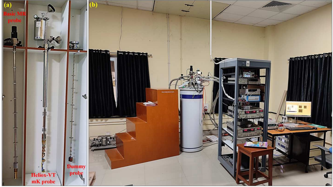
FIGURE 3.65: (a) Three probes/inserts for transport measurements using Oxford Teslatron system, (b) Image of the Oxford laboratory at SNBNCBS.
