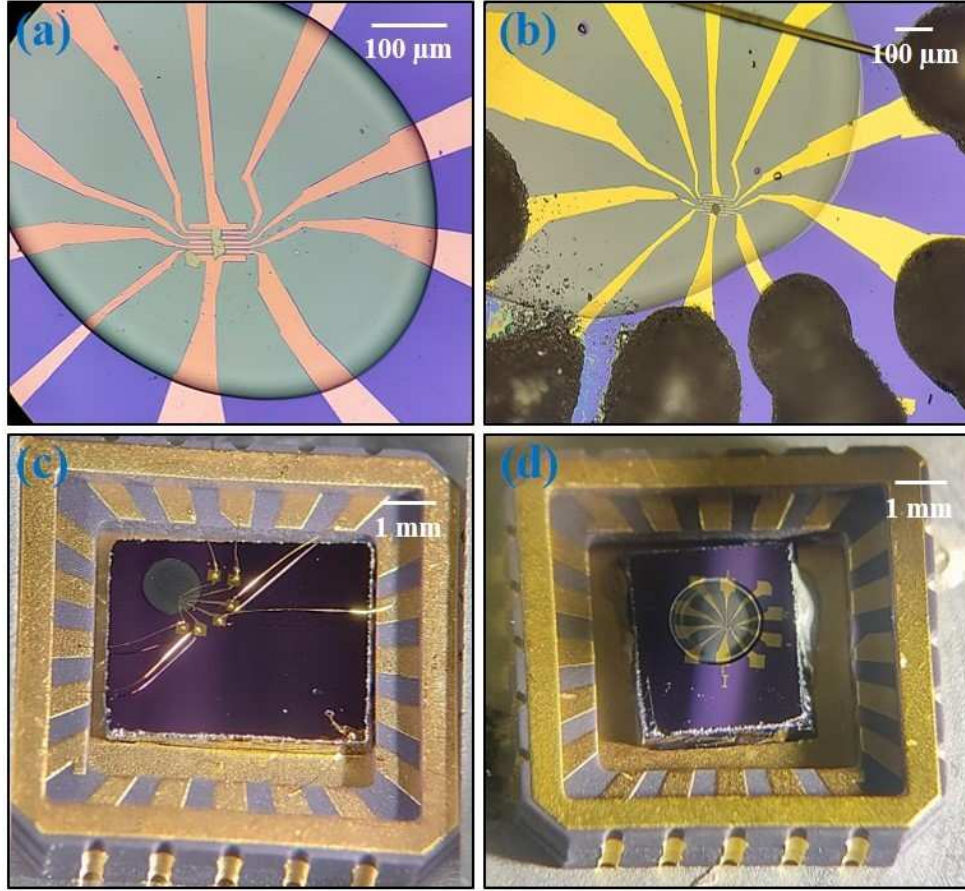
FIGURE 3.29: (a), (b) PMMA-coated flakes transferred on top of pre-patterned gold electrodes. (c), (d) PMMA-coated devices bonded and mounted in 20-pin LCC chip carriers.
