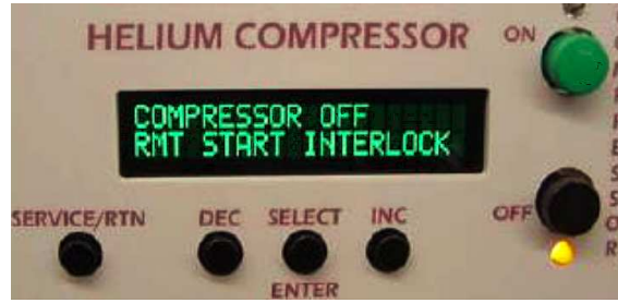
FIGURE 3.34: Compressor display panel [276] after powering on
