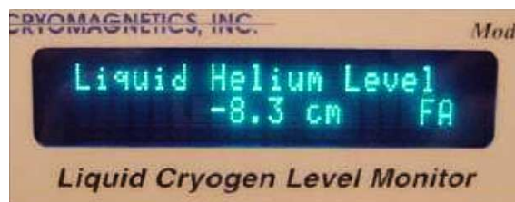
FIGURE 3.36: Typical view of the liquid level monitor’s display panel [276].
