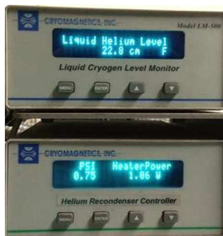
FIGURE 3.38: Display panel of the compressor package after starting LHe production.
