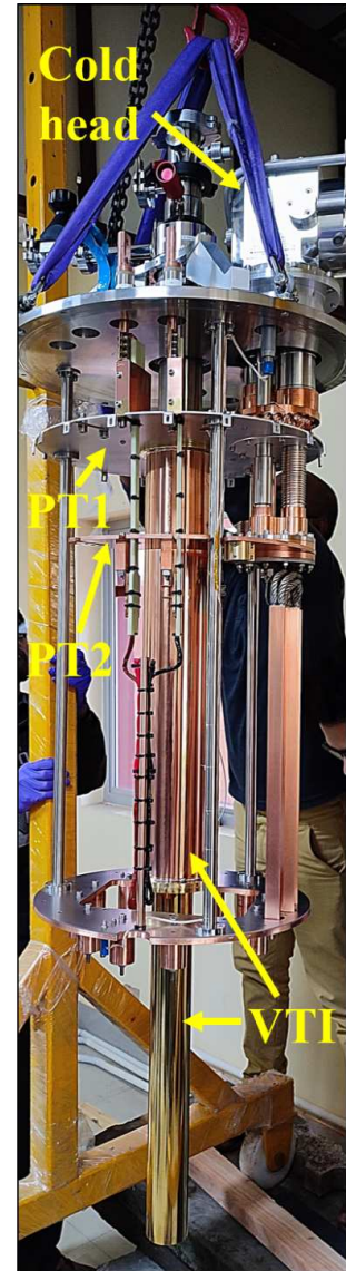
FIGURE 3.56: Internal structure of the Oxford cryostat during installation.
