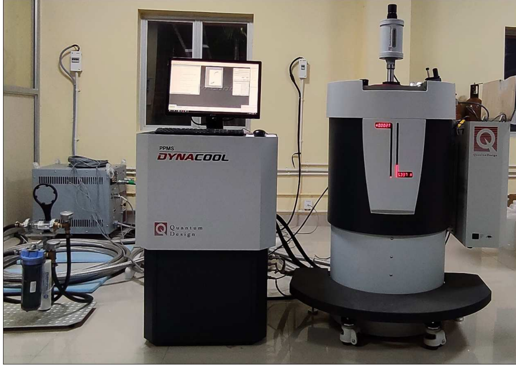
FIGURE 3.50: PPMS setup image with VSM option at SNBNCBS
