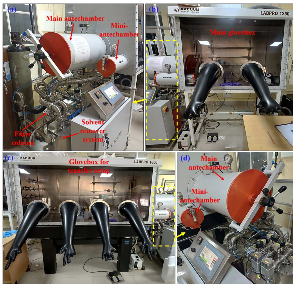
FIGURE 3.67: Image of the glove-boxes in our lab at SNBNCBS (a), (d) Image indicating the different components of the (b) main glovebox and (c) glovebox for transfer setup.
